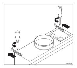
■ Loosen the screws of the fixing brackets on the top of the appliance.
